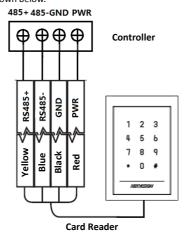
Figure 3-4 Wiring for RS-485 Communication Mode
