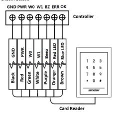
Figure 3-5 Wiring for Wiegand Communication Mode
